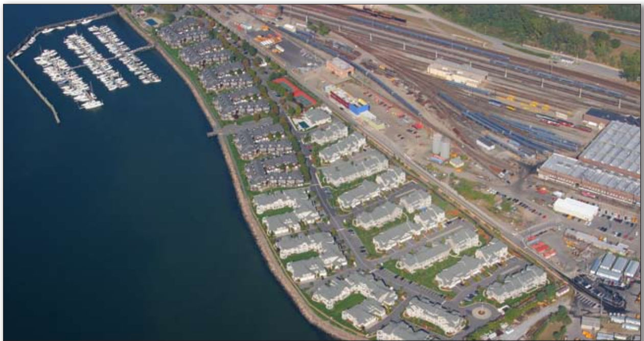
This development includes several examples of poor riverfront development practices: inadequate building setback, repetitious building architecture, white exteriors, unvegetated shoreline, lack of open space, and uninviting public access.
