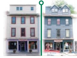
Removal of the vinyl siding has provided functional and aesthetic advantages to this façade. The original siding has more depth of detail and gives more impact to the architectural quality of the building. The roof top dormers were also replaced with more appropriately designed dormers that significantly increase the buildings stature and financial value.
