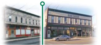
Refurbished windows, replacement of doors, a restored mid-cornice, powerwashed facade and new painting has transformed this important building into a shining example for the community to admire.
